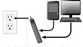
Insert the MMS370 into a utility outlet with the Surge and Grounded LED lights facing up. Next, connect your devices to the MMS370. Verify the Red LED is activated. If so, the MMS370 is actively protecting your equipment. If off, then the MMS370 has an internal fault or has absorbed a large-enough spike to be damaged and should be replaced. The Green Grounded LED indicates a proper grounding. If unlit, the circuit has improper earth-ground and should be checked by a qualified electrician.
