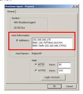
4. Go to SentryHD's SNMP Trap page and input the IP address of the MM ShutdownAgent's Host Server into the SNMP Trap table as the Target IP. Select the MM ShutdownAgent for the Event Level and UPSv4 as the Trap MIB.
