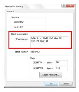
2. Login to the MM ShutdownAgent input the Host Server IP address into the Source Trap IP and the trap port to receive the SNMP trap from SentryHD.
