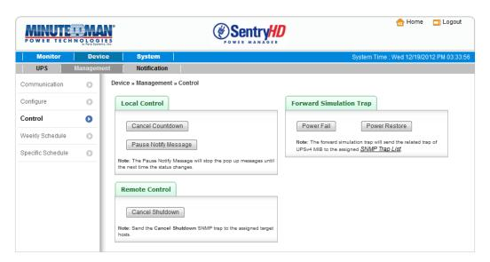
**Local Control:** Press the "Cancel Countdown" button during the countdown shutdown process to stop the countdown. Press the button again to resume the shutdown process. In addition to selecting the Resume Countdown menu item to continue the countdown process, it will also start a new countdown process.
