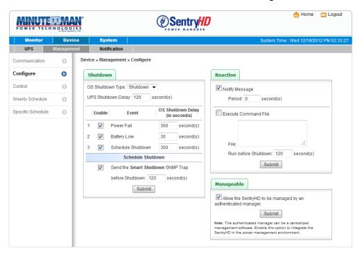
**Shutdown:** Select the Shutdown Type to determine the best way to shutdown the operating system. The options are Shutdown, Power Off and Hibernate. The default value is Shutdown. Select the event that will trigger the Shutdown action and enter the amount of time it will take the OS to shutdown. If the event recovers during the countdown then the shutdown process will be cancelled, the host will not be shutdown.
