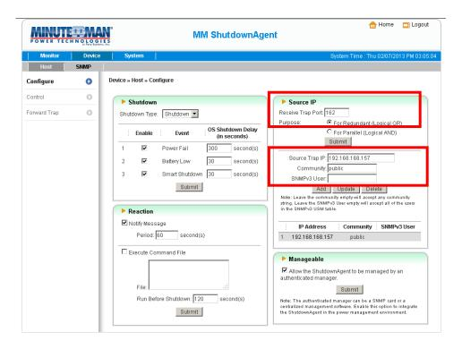
3. Open the MM ShutdownAgent property menu from Windows task bar to get the IP address of the Host Server.
