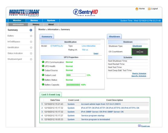
**Identification:** Displays the information about the UPS's Model, Type and VA Rating. **UPS Properties:** List the major UPS properties for monitoring the UPS health, output and battery status.
