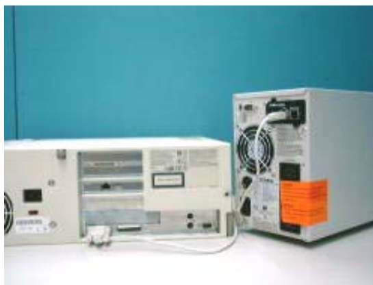
Figure 2-2: Serial cable connection of SNMP-SSL
