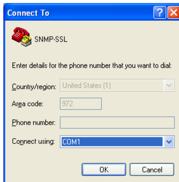
Figure 2-5: Select Direct to COM port connection
