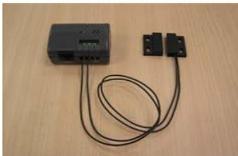
3. Attach the sensors to the door and doorframe.
