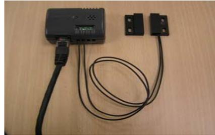
5. Verify that the SNMP-SSL card has a network connection and is powered on.
