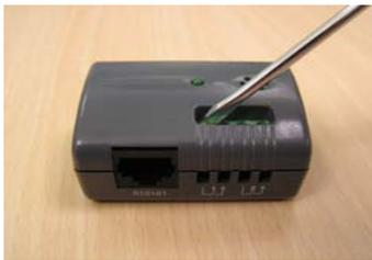
2. Connect the wires of SSL-DOOR to the SSL-EMD Alarm-1 and/or Alarm-2, and then tighten the screws.
