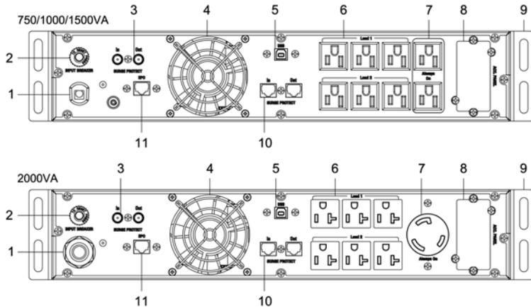
1. The input power cord is for connecting the UPS to utility power. **NOTE:** The AC wall outlet shall be near the UPS and easily accessible.
