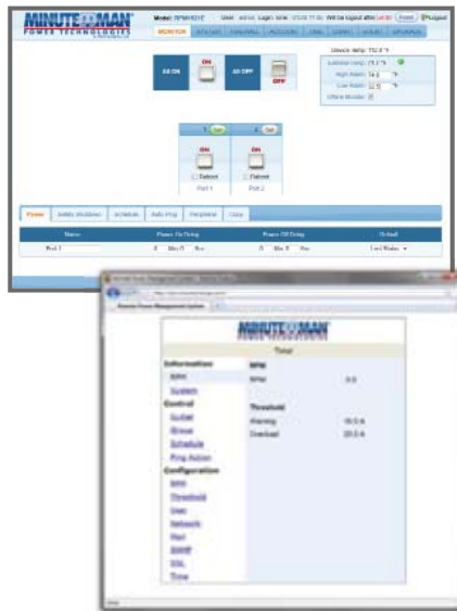
RPM1521E (above) and RPM 8 and 16-port interface main screens
