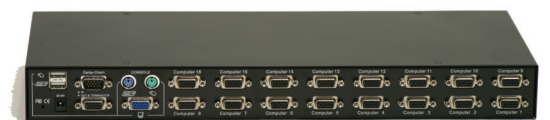
Rear of 16 port USB-PS/2 KVM with On Screen Display and No Delay Switching - model MMAUSB1680SD
