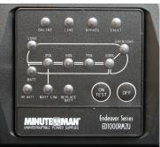
that measures both connected load capacity and battery runtime capacity. The LED panel is designed so that it can be oriented vertically or horizontally depending on the installation format of the UPS.
